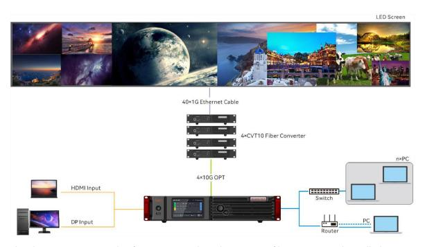
This diagram is an example of two input cards and one 4x10G fiber output card installed on an MX2000 ROE. The actual application may vary.
