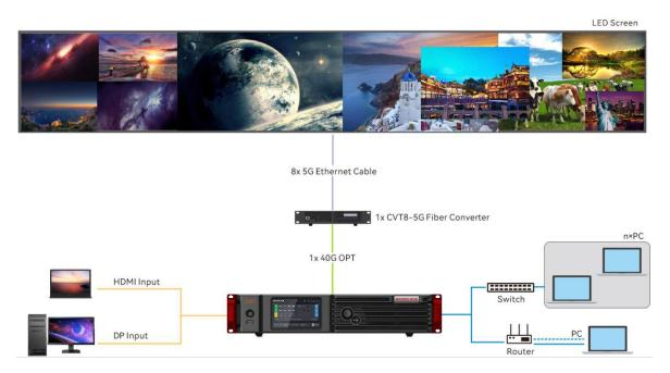
This diagram is an example of two input cards and one 1x40G fiber output card installed on an MX2000 ROE. The actual application may vary.
