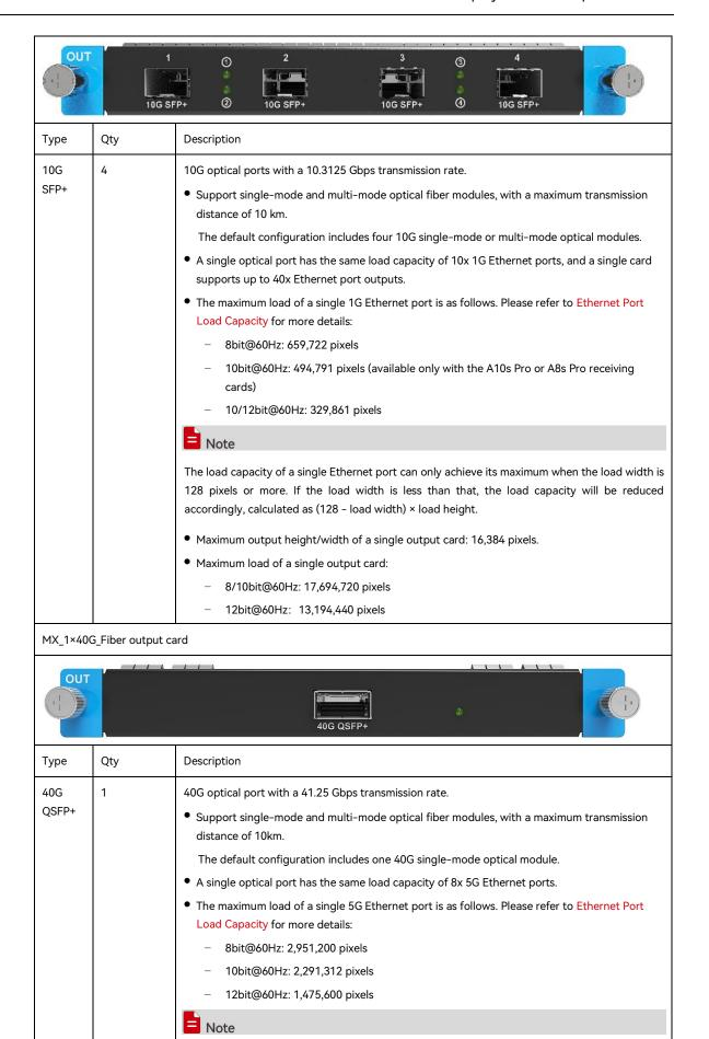
The load capacity of a single Ethernet port can only achieve its maximum when the load width is
